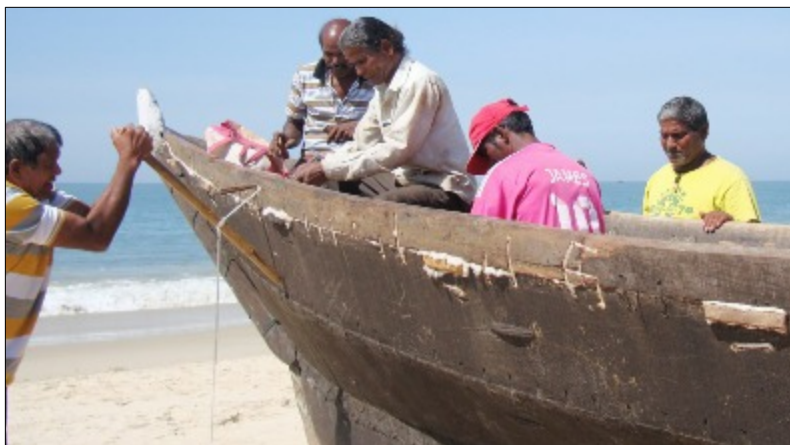
Figure 18. Assistant uses force on a lever to tighten a stitch. Fish Road. Author.
