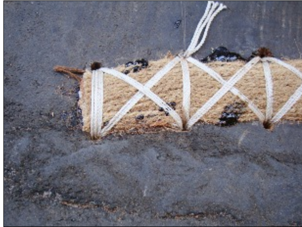
Figure 17. New stitches inboard; hammering has squeezed out chandrus . Above, an old seam. Fish Road. Author.
