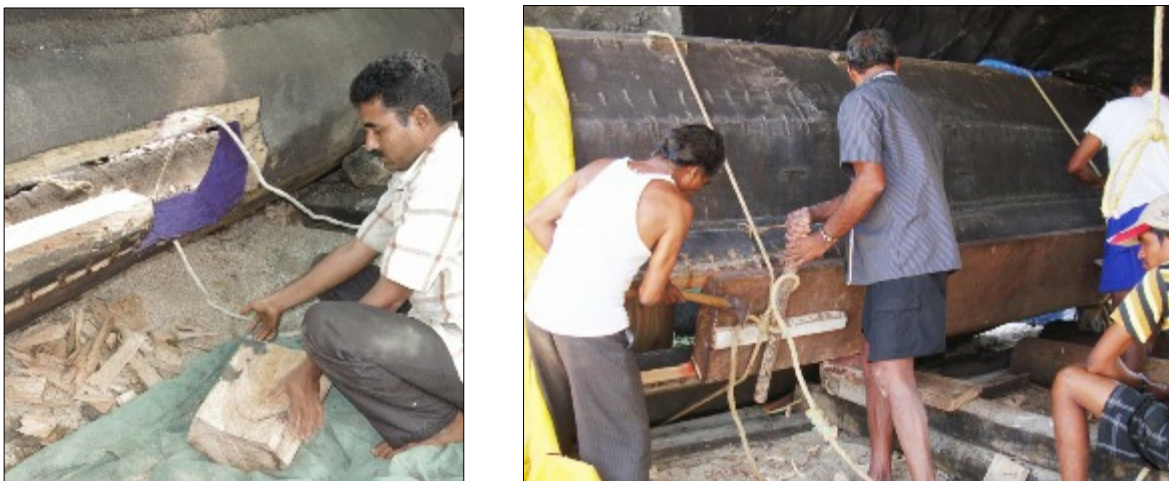
Figure 14 Repair to the underbody of a pirogue involves offering up new work numerous times: a) Siridau; b) Benaulim. Author.
