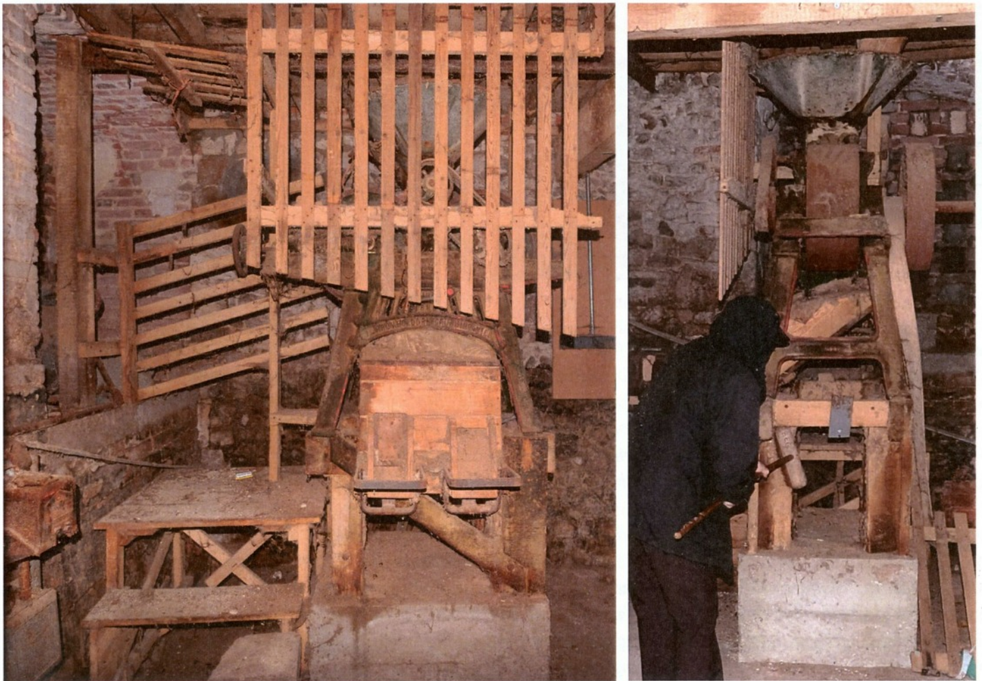
Fig 11. A long-disused mill used to crush the corn for livestock rations in Butley Abbey's Great Barn. (photo: Paddy O'Beirnes)
