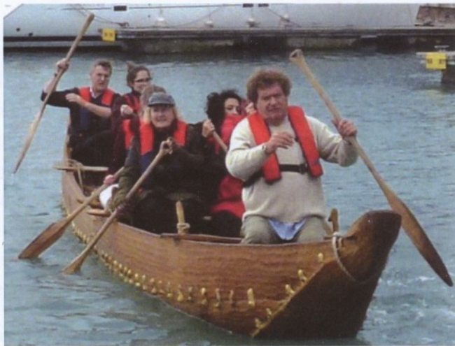
A half-size reconstruction of the boat was trialled in Dover Harbour. Beeswax sealed the stitch-holes
