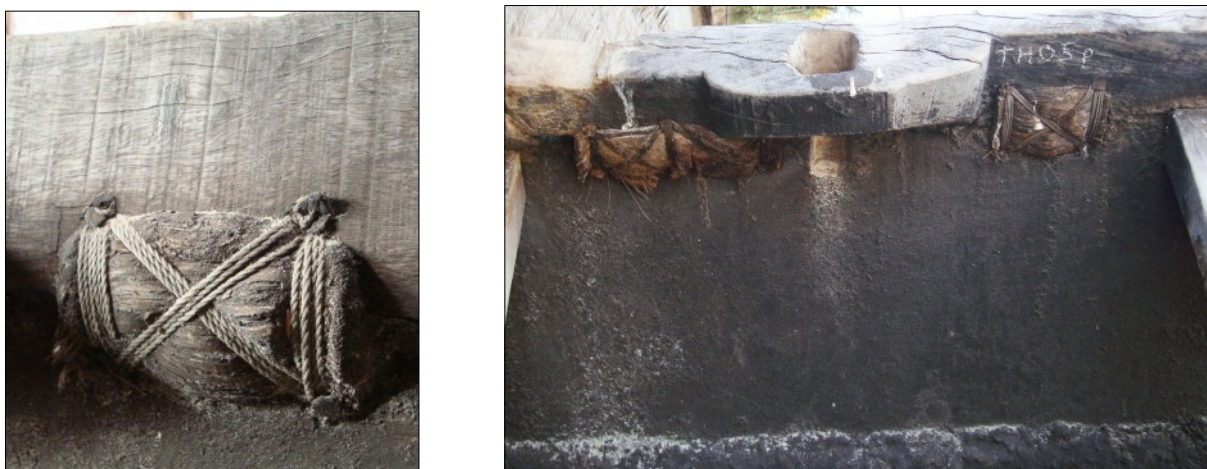
Figure 10. a) wedged stitch pad. Colva; b) narrow sheer strake with carved thole and thole-pin wear, flanked by paired padded stitches. Benaulim. Author.
