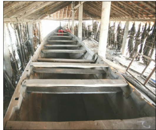
Figure 8. In the bow over the thwart-beams large pirogues have thwarts rabbeted on the sheer: a) 14.2m long. Siridao; b) laid-up pirogue 13.4m long showing thwarts and absence of internal stiffening. Arossim. P. O'Beirnes.
