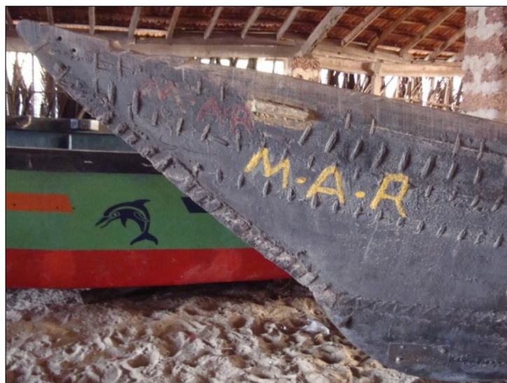
Figure 7. a) new stem-cap with only five stitches securing it. Velsao Danddo; b) old stem minus its stem-cap, revealing closely oversewn hood-ends. Sernabatim. Author.
