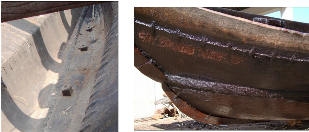
Figure 4. a) barely visible stitches inboard between the underbody and garboard. Bolts fasten a false-keel along the centreline of the underbody. Fish Road; b) well-maintained two-strake pirogue with false-keel attached by stitches. Cova. Author.
