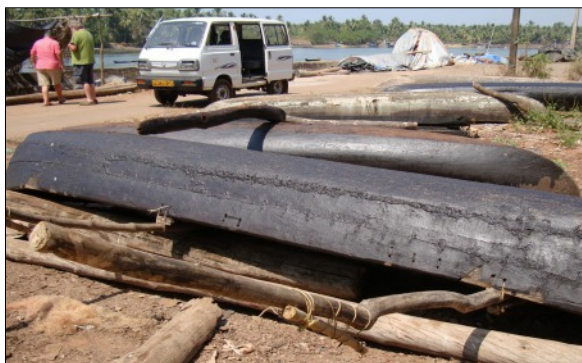
Figure 2. Monoxyllous craft used on Goa's rivers. They are so heavily coated in dikh that sewn portions are difficult to detect: a) upturned with booms still attached. Assolna; b) under repair on the slip at Cavelossim. Author.
