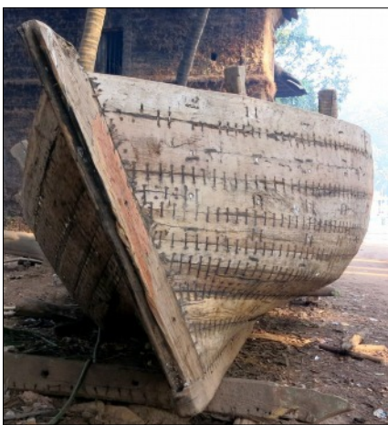
Figure 24. Sewn wooden dredgers used on Goa's rivers: a), b) 12m long under repair at Volvoi Ferry; c) beached near Keri. Author.
