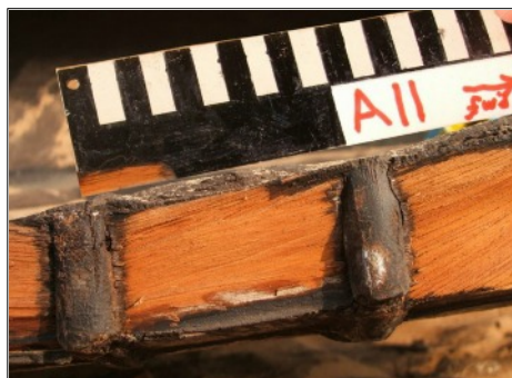
Figure 21. Fracture shows encrusted surfaces and wedges in stitch-holes impregnated with dikh . Benaulim. Author.
