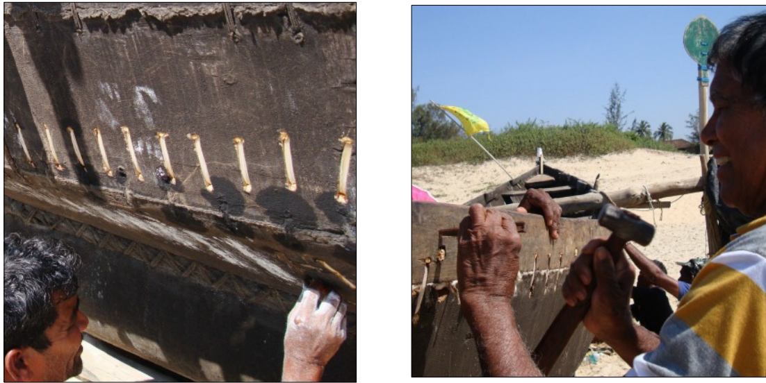
Figure 12. Outboard: a) grooves span a new split and an old seam. The surface is made good below with hand-applied chunam ; b) ends of wedges are trimmed and battered. Fish Road. Author.
