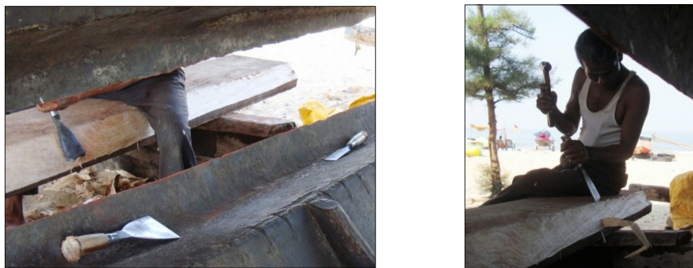
Figure 13. a) the three edge-tools used by a master boatbuilder; b) shave with a curved blade achieves a fine finish. Benaulim. Author.
