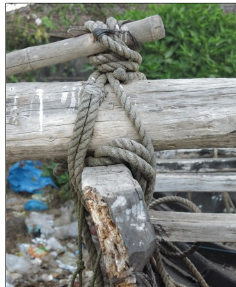
Figure 11a) Outriggers are set aft of midships and fastened by six quick-release onns . P. O'Beirnes. 11b) Extremity of float shows level of normal immersion. Velsao Daddo. 11c) onn on a derelict. Siridao. Author.
